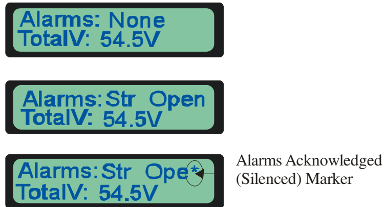
Figure 15: Variations of the Alarm Display
